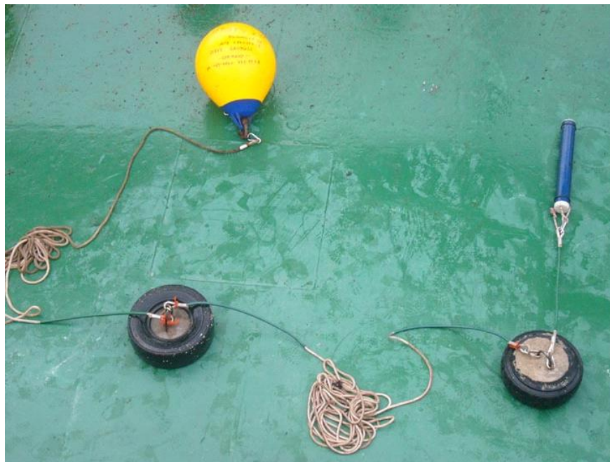
Fig. 8: T-POD mooring system with two anchor blocks (tyres with concrete).
