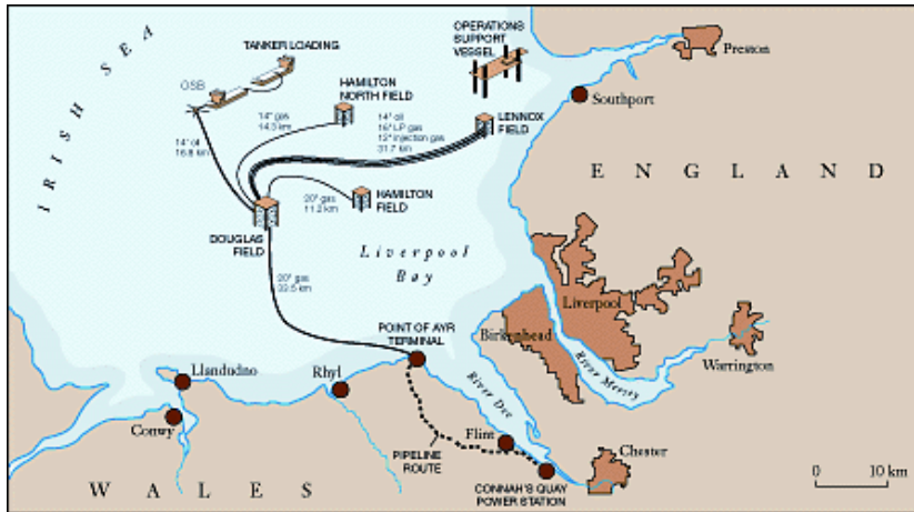
Figure 6.11: Offshore oil and gas facilities in Liverpool Bay (Courtesy of www.ipicea.org)
